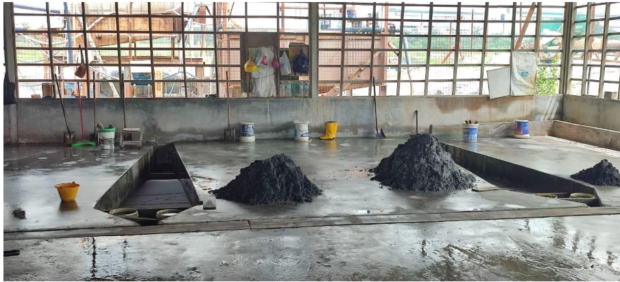
The washed tin ore, which would be further refined using magnetic separators
