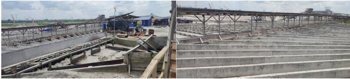
The Palong to separate the tin ore, which sinks and is contained in the “rifles”
