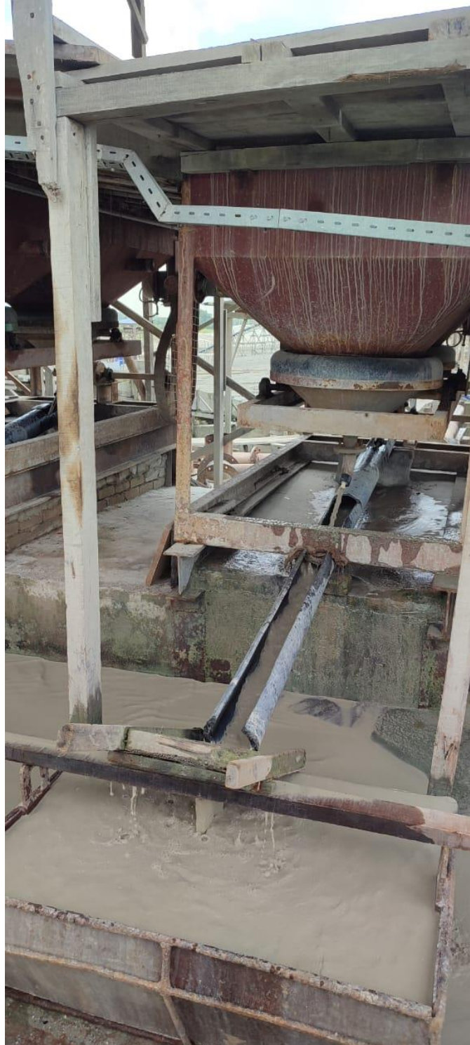
A jig which uses a certain frequency to separate the minerals
