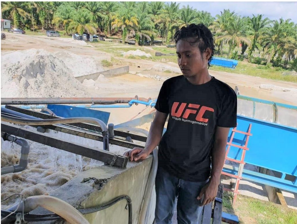
Palong to separate the silica from the lower grade sand.
